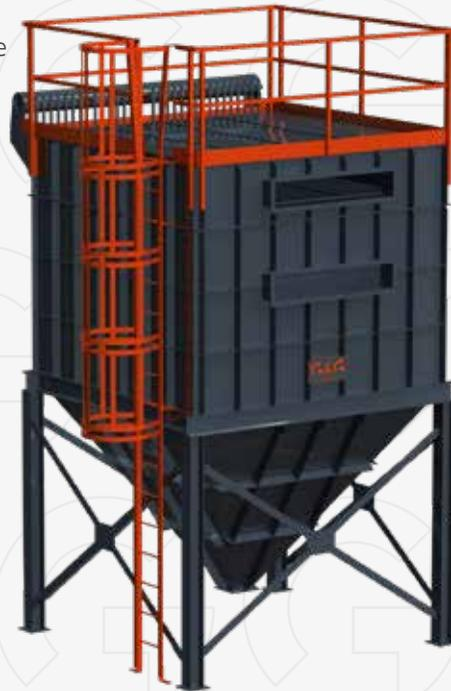
The filtration device is thermally insulated over the entire casing and is equipped with an electric heating cable for tempering the filter housing and preventing condensation of flue gases at the moment of starting or stopping the boiler at a low flue gas temperature.
